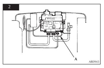
2.3 Loosen main injector nut on airbox and disconnect from injector, see diagram 3, A.
